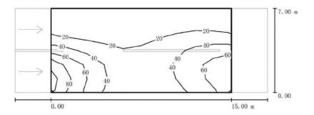
Remarks: Symmetrical lamp arrangement; pole spacing is recommended to be three times longer than lamp height.
