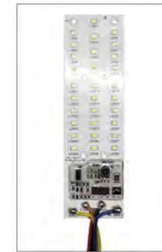
Lens controller + highlight lamp bead + aluminum substrate
